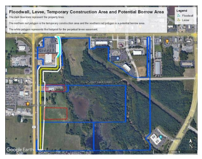
Figure K:2-1. Map of Levee and Floodwall for Flood Risk Reduction
